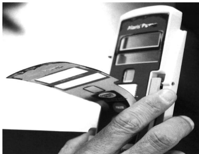
**Figure 1.** Alaris Pump Module Model 8100, showing overlay separation. Image courtesy of Carefusion 303.
